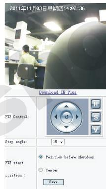
【PTZ Control】 : : resetting; : upward/downward scanning; : stopping; : horizontal scanning; you can control the camera turn direction.
