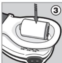
3. Remove the depleted battery.
