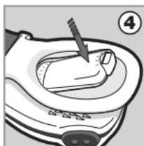
4. Insert the new battery, ensuring that the polarity is correct (align the positive end '+' of the battery with the '+' symbol in the battery housing, as indicated). Replace the Battery Cover and ensure that it is correctly closed.
